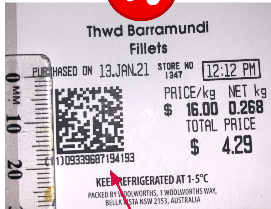
Incorrect no Quiet Zone (white space) around the barcode
