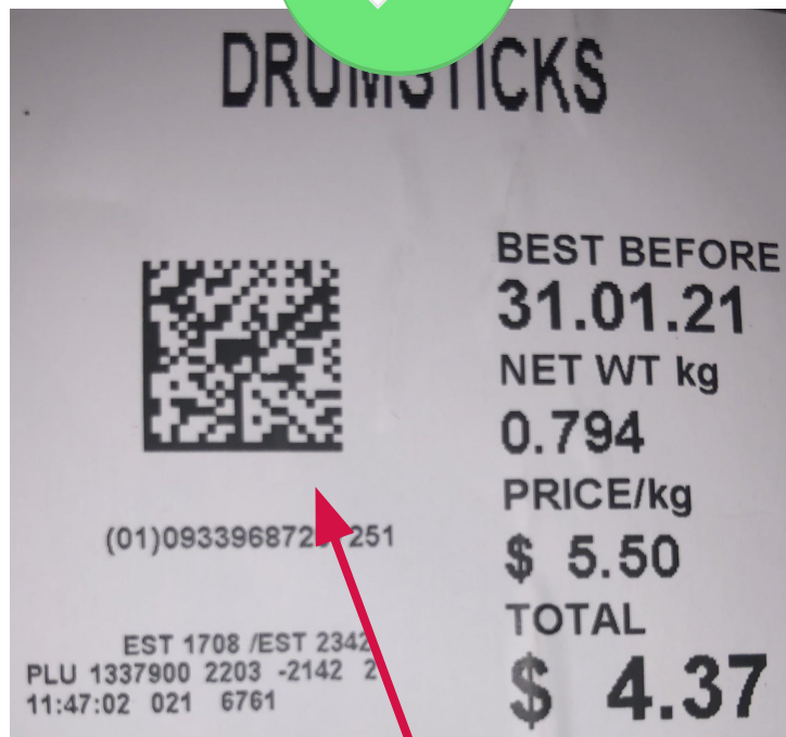
Minimum Quiet Zone (white space) around the barcode >1.3mm
