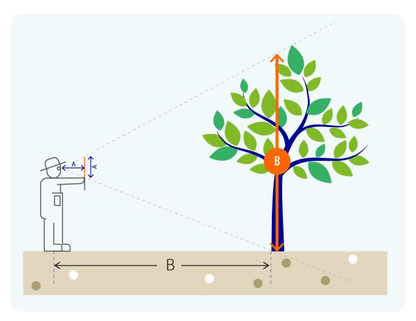
Figure 8. How to measure the height of a tree without a laser measuring tool
