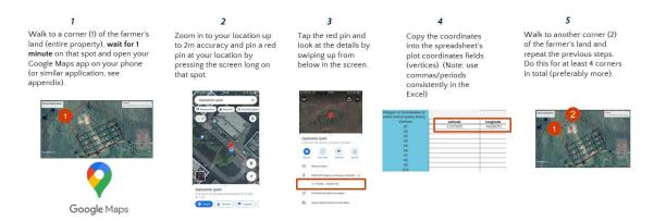
Figure 4. Step-by-step approach to determine coordinates
