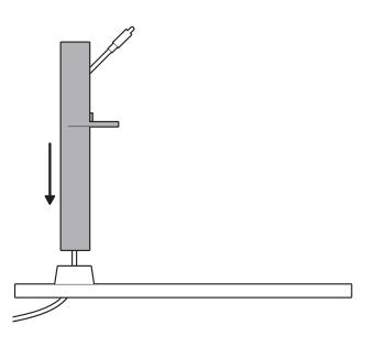
Tighten the tapping screws included with your camera to secure.
