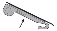
**NOTE:** If installing under cold conditions, lay the holder on your dash and turn your vehicle's defroster to the highest setting to prime your windshield and the holder adhesive for application. Install once the windshield and holder are warm to the touch. For best results, wait 24 hours for the adhesive to bond fully before installing your camera into the holder.
