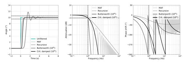
The graphs above show a comparison between the *Moving Average Filter (MAF)*, a *Simple Recursive Filter* and both a 10<sup>th</sup> order *Butterworth* and *Critically Damped Filter*, all having a cut-off frequency of 1 Hz.
