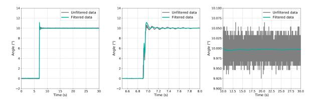
The graphs above show an exemplary trace of measured data including signal noise upon a steep 10° step as well as the filtered signal using an (adaptive) *Kalman filter*. While the left graph shows the complete curves, the middle and the right graphs depict zoom-ins into specific time and angle ranges to illuminate special filter characteristics.
