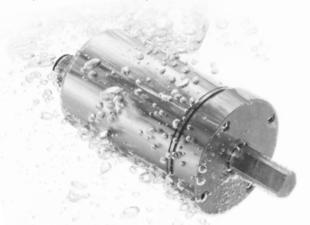
IXARC rotary encoders can provide up to IP69K protection class. The design of stainless-steel housing and flange is available, which can protect encoder against the corrosion from gas and dust. The heavy-duty version encoders can withstand shaft loads of up to 300N and offer a shock resistance of up to 300g.
