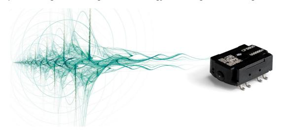
Wiegand sensors offer magnetic sensing without the need for any external voltage or current to be applied. The material properties of the sensor mean that consistent pulses are produced every time the magnetic field polarity switches. In addition to magnetic sensing, ultra-low power electronics can be powered by harvesting the energy of a single pulse, or successive pulses can be stored to offset energy demand of circuits.
