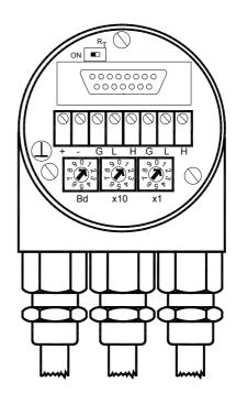
A termination resistor is integrated in the connection cap. The resistor must be switched on if the encoder is connected at the end or at the beginning of the bus. Separation of Bus In and Bus Out signals if termination resistor is activated. Resistor:
