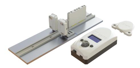
UBITO WINK is a DevKit which is made to provide developers with the essential components for creation of energy-autonomous devices that can detect real-world events involving moving magnetic fields and transmit measurements wirelessly to a remote monitoring system.
