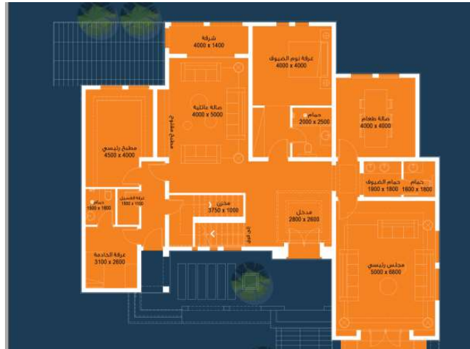
Figure 1: An example of what you would see in a Concept Design package. this drawing shows a basic floor plan to show how the space is being used (i.e. horizontal relationship).
