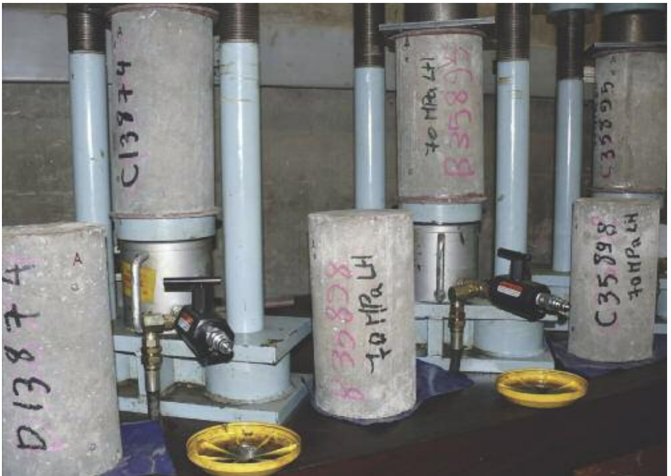
Figure 2: CLH - Creep and drying shrinkage testing of concrete after 3 months
