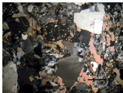
Fig. 11. Cement of sparitic calcite in Pietra Serena extracted from the Gonfolina quarry (image in thin section, under optical microscopy in transmitted light, xpl).
