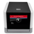
Confirm the Chromium Single Cell A program shows on the screen and press the play button to start the run
