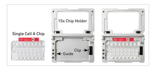
c) Close the hinged lid of the 10x Chip Holder. After loading the Chromium Chip, the 10x Chip Holder should lay flat on the bench top with the lid closed.
