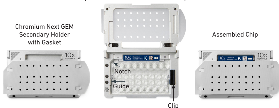
Chip in Chromium Next GEM Secondary Holder
