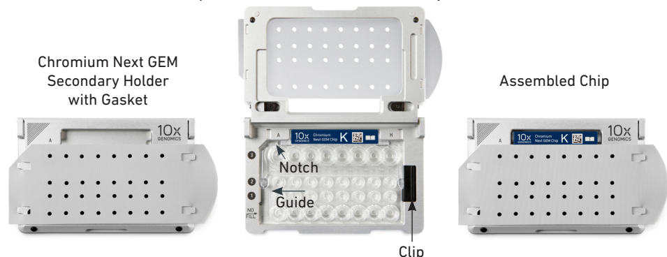
Chip in Chromium Next GEM Secondary Holder
