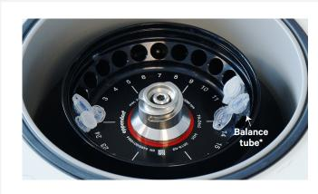
\*Caps of tubes are angeled toward the balance tubes to prevent them from turning outward due to the centrifugal force.
