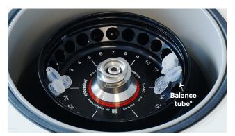
\*Caps of tubes are angeled toward the balance tubes to prevent them from turning outward due to the centrifugal force.
