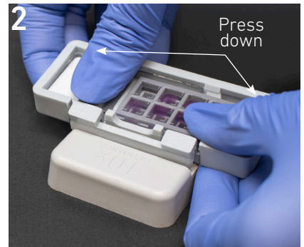
Push Insert Clip along the ridge & press down
