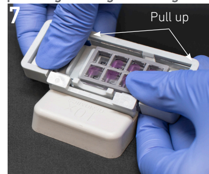
7 Remove Slide Cassette while pressing slide against the gasket
