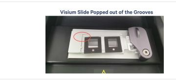
• **Debris is present** on the Tissue Slide Stage or Visium Slide stage: see System Maintenance section to clean the area.
