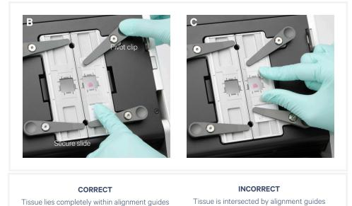
**d.** If only one tissue on one slide will be loaded, use a blank slide for the second position on the Tissue Slide Stage.
