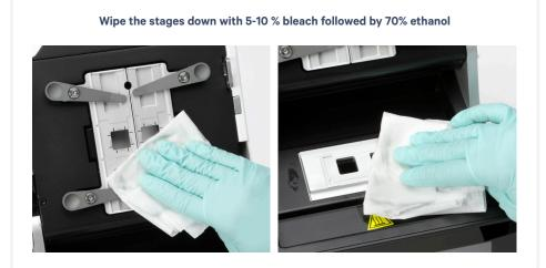
**d.** Close the lid (clicking sound indicates closure). Wipe down the base and lid of the instrument.
