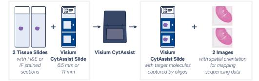
Further optimization of Visium experiments can be achieved by prescreening tissue sections using standard histological techniques to find biologically significant sections, then using the CytAssist instrument workflow to precisely align those sections within the Visium Capture Areas. Using Visium Cytassist, analytes from up to two FFPE tissue sections can be captured on CytAssist specific slides in less than one hour per run.
