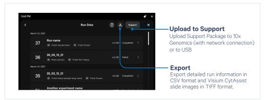
\*Idle time data are only instrument-specific logs that are not related to runs. The data are exported with the Support Package. During First Time Use (FTU) set up, it can be accessed using the help icon on the top right corner of the screen.
