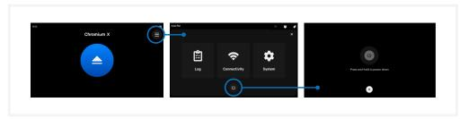
Power off the instrument by tapping the power icon at the bottom of the menu options screen. The system will go into a soft power down (screen is dimmed and displays time and name of instrument).
