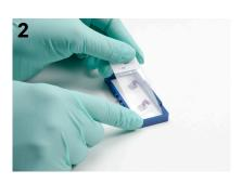
Securely combine gasket with top half of cassette until the gasket snaps into place.
