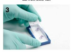
Open cassette by continuing to lift clip upward. If slide sticks to gasket, continue to apply even upward pressure to separate slide from gasket
