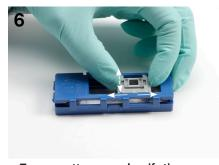
Turn cassette over and verify tissue area of interest is within gasket. DO NOT move gasket once cassette is closed. If necessary, open cassette and recenter gasket.
