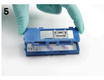
Apply even pressure on top of cassette until it clicks shut. Verify that clip is completely secured over hinges.
