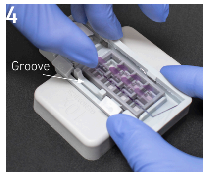
Lift slide at Slide Cassette groove
