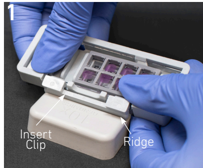
Position Slide Cassette along alignment tool ridges
