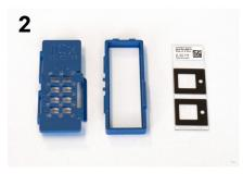
Press slide down into grooves of the bottom half of the cassette until it sits firmly in place
