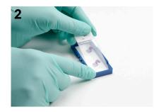
Securely combine gasket with top half of cassette until the gasket snaps into place.
