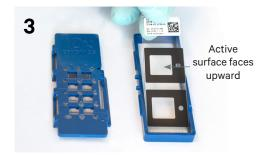
Place upper and lower halves of cassette, and Visium slide, directed upward on bench
