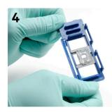
Adjust gasket such that gasket is over the tissue area of interest. The 6.5 mm gasket can be adjusted horizontally as well as vertically.
