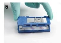
Apply even pressure on top of cassette until it clicks shut. Verify that clip is completely secured over hinges.
