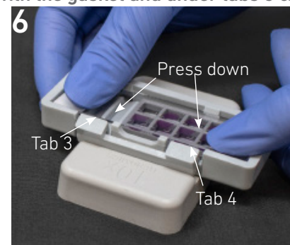
Press slide down until it is flush with the gasket and under tabs 3 & 4
