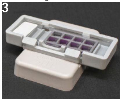
Slide Cassette Sits securely on alignment tool
