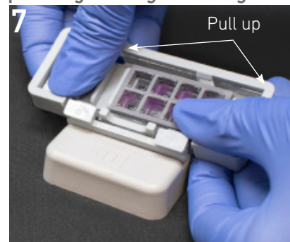
Remove Slide Cassette while pressing slide against the gasket
