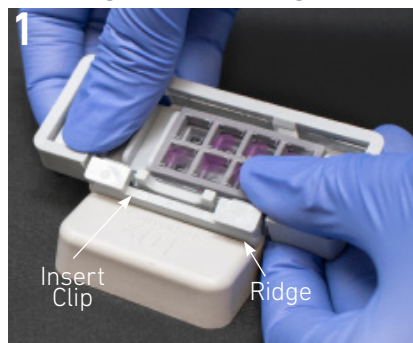
Position Slide Cassette along alignment tool ridges
