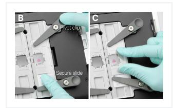
**d.** If only one tissue on one slide will be loaded, use a blank slide for the second position on the Tissue Slide Stage.
