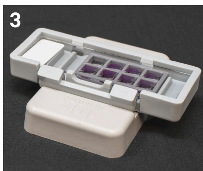
Visium Cassette sits securely on alignment tool
