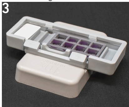
Slide Cassette Sits securely on alignment tool
