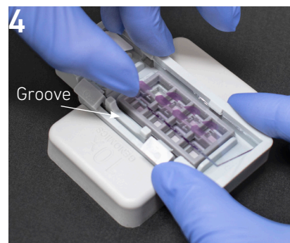
Lift slide at Slide Cassette groove
