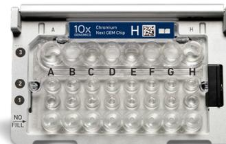
Recovery well G indicates a reagent clog. Recovery well C and E indicate a wetting failure. Recovery wells B, D, and F are normal. Wells A and H contain 50% Glycerol Solution.
