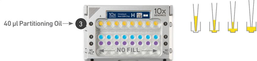
**!** Attach the gasket and run the chip in the Chromium Controller **immediately** after loading the Partitioning Oil.
