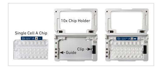
b) Close the hinged lid of the 10x Chip Holder. After loading the Chromium Chip, the 10x Chip Holder should lay flat on the bench top with the lid closed.
