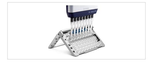
b) When transferring the GEMs from the Chip A Single Cell after the Chromium Controller run into the tube strip or plate (on a chilled metal block resting on ice), the pipette tips should be positioned against the side walls of the wells as shown for a plate below.
