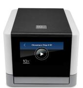
Confirm the Chromium Chip A Single Cell program shows on the screen and press the play button to start the run
