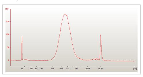
b) OR Run 1 µl of sample at 1:10 dilution on the Agilent TapeStation High Sensitivity D1000 ScreenTape for qualitative analysis. Traces should resemble the overall shape of the sample electropherogram shown below.
