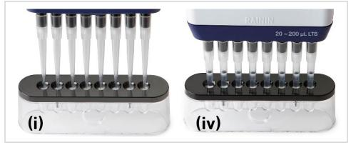
c) If the required volume of beads cannot be recovered, place the pipette tips against the sidewalls of the Gel Bead Strip wells and slowly dispense the Gel Beads back into the strip. Take care not to introduce bubbles into the wells and verify that the pipette tips contain no leftover Gel Beads. Attempt to withdraw the full volume of beads again by pipetting slowly.
