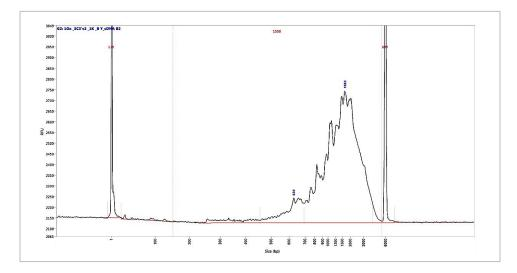
b) Run **2 µl** of Post Library Construction sample on the Fragment Analyzer Automated CE system for qualitative and quantitative analysis. Traces should resemble the overall shape of the sample electropherogram shown below.
