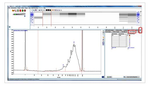
e) Toggle the Show Results icon on the upper right side of the screen and select Smear Analysis tab to display the concentration and the average size of the analyzed sample.
