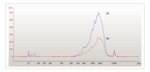
If the input cells are particularly RNA-poor (<1pg total RNA/cell), it may be necessary to run 1  $\mu$ l of undiluted product (trace b). Lower molecular weight product (35 – 150 bp) may be present. This is normal and does not affect sequencing or application performance.
