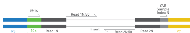
Figure 1. Schematic of final library construct of a Chromium Single Cell ATAC library. The 10x Barcode (16 bp) is sequenced in the i5 index read and the Sample Index N is sequenced in the i7 index read. The accessible chromatin insert is sequenced in Read 1N and Read 2N.
