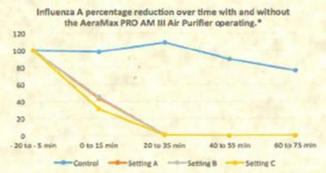
\*Results represent the average of n=3 runs. Device settings A: ionizer ON and filter low speed; device setting B: ionizer off and filter at low speed; device setting C ionizer og and filter at high speed.
