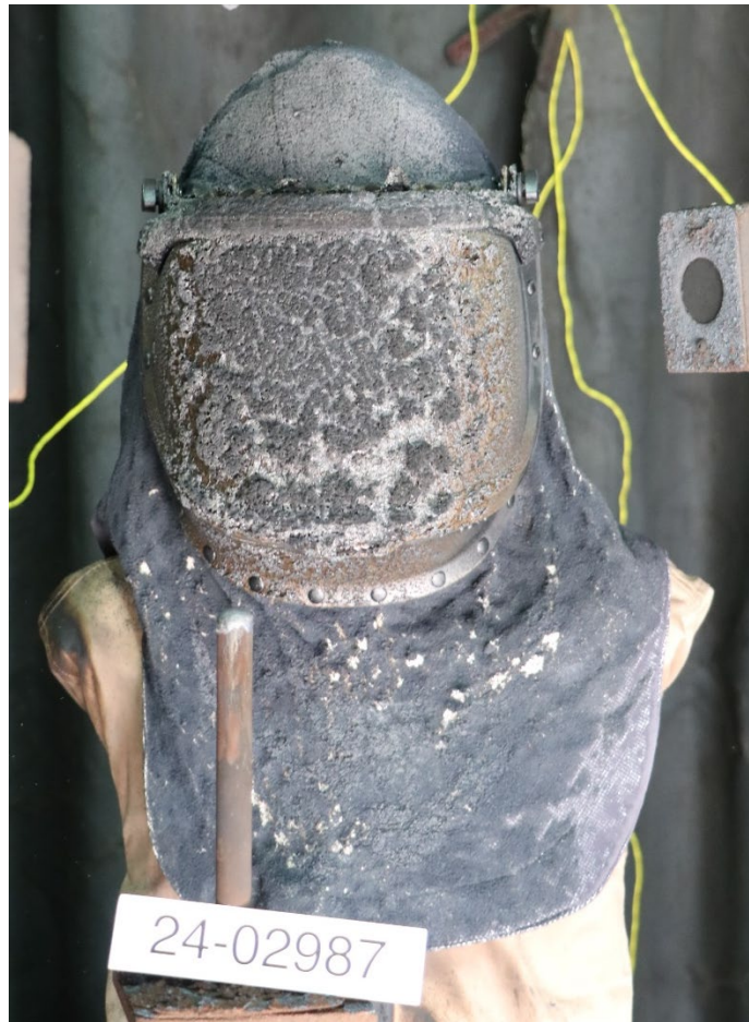
Figure 6-4: Sample after the arc exposure, 49 cal/cm 2 .
