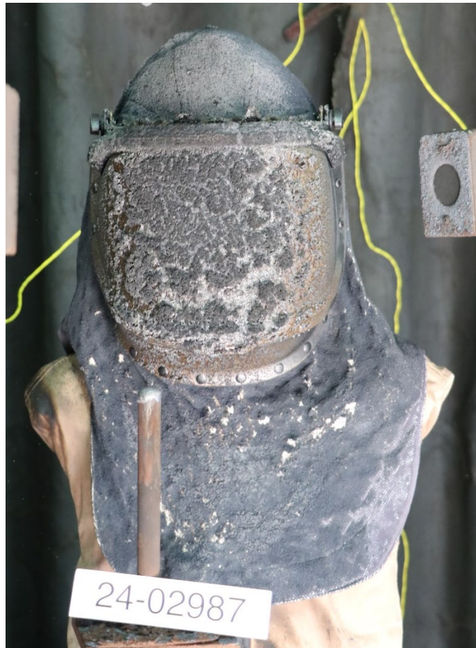
Figure 6-4: Sample after the arc exposure, 49 cal/cm 2 .
