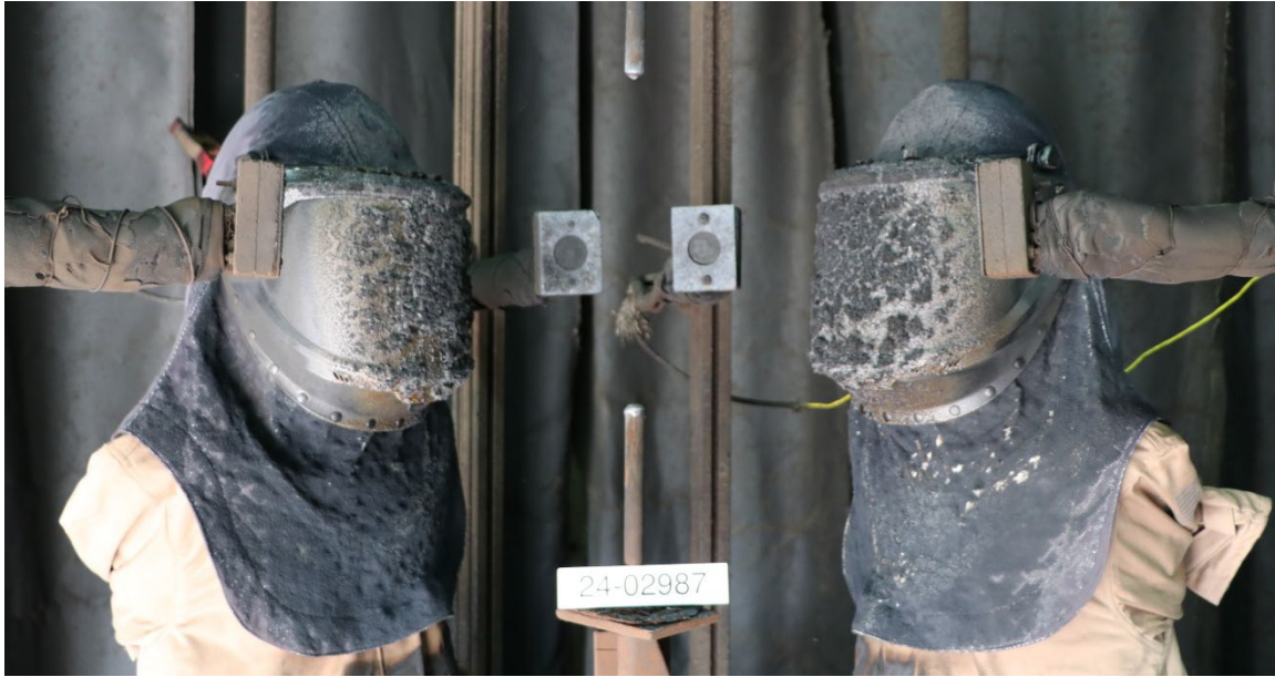
Figure 6-3: Samples after the arc exposure, 44, 49 cal/cm 2 .
