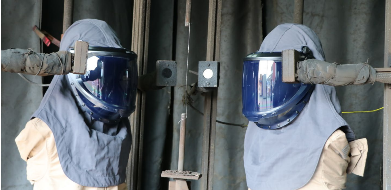
Figure 6-1: Samples as tested before the arc exposure.
