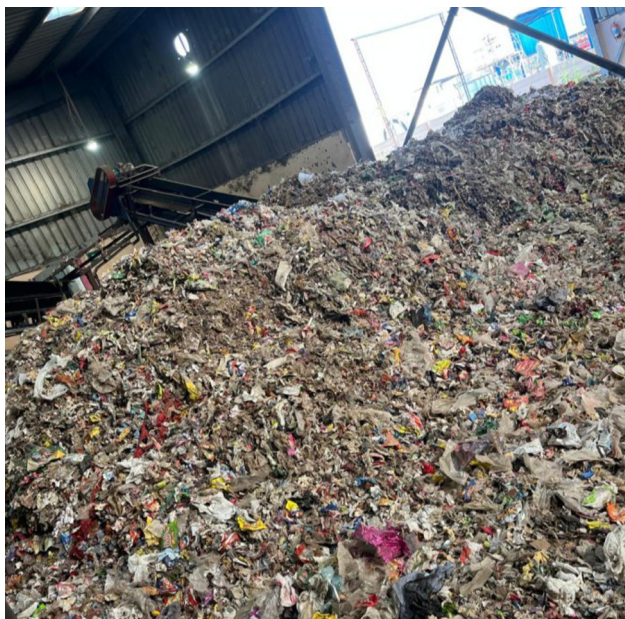
Fig.1. Photograph of MSW-RDF received at site.
