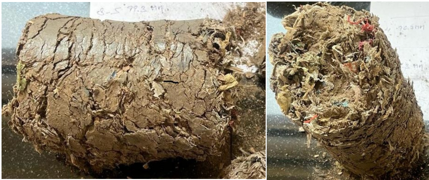
Fig. 6. Photograph of the MSW Briquettes.
