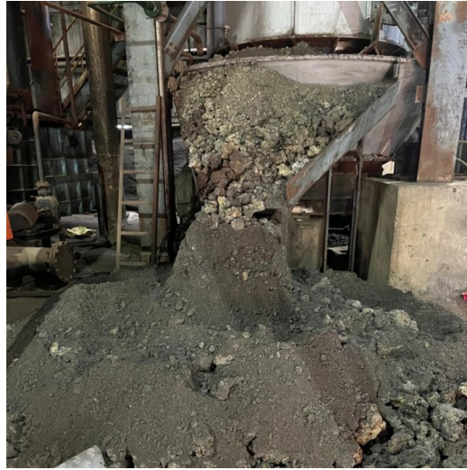
Fig. 11. Photograph of the ash collection from gasifier.
