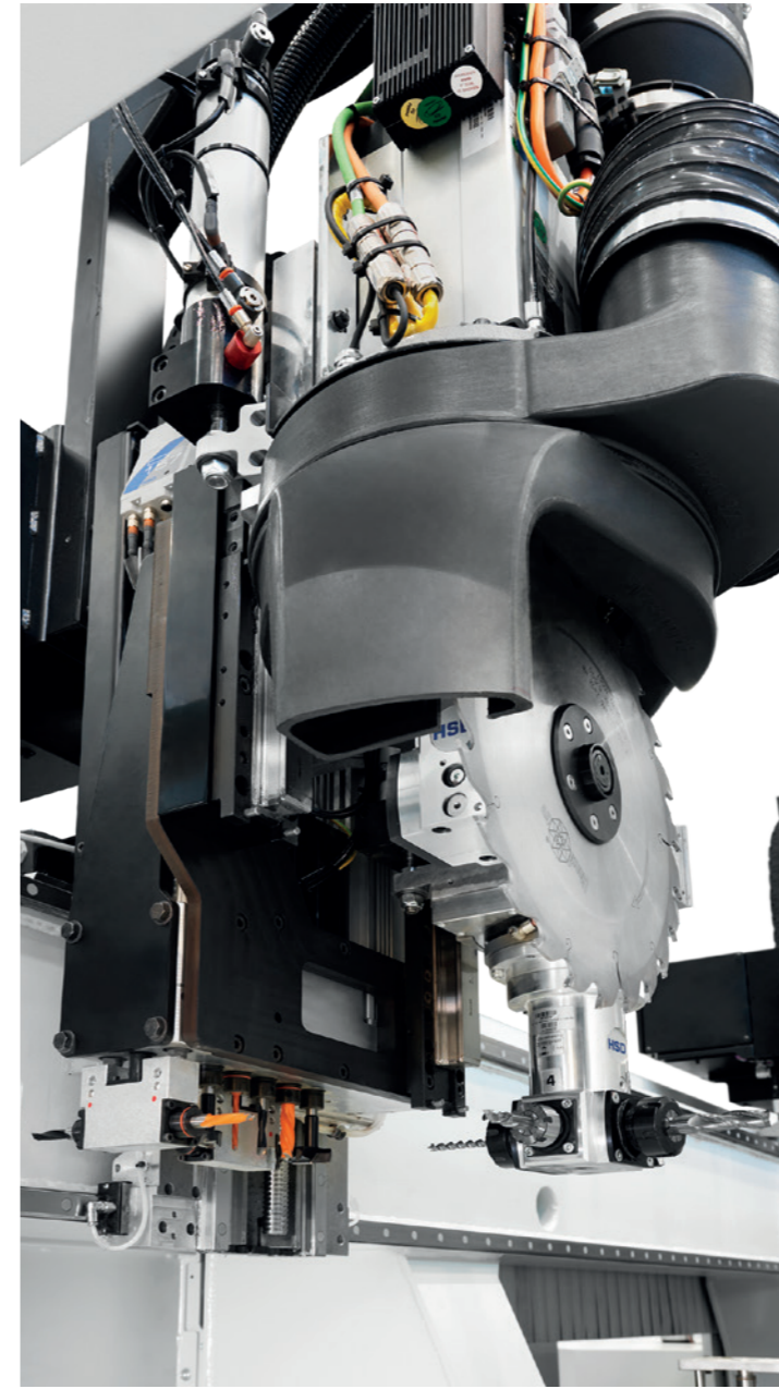
The Rover A Plus can be configured with a five-axis and/or four-axis milling unit with maximum power of up to 16.5 and 19.2kW
