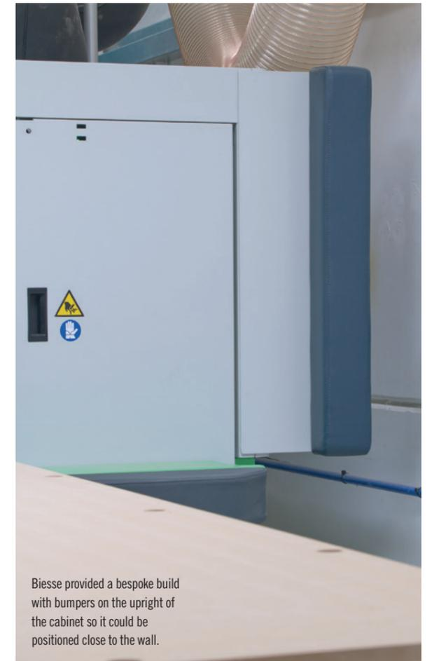
Biesse provided a bespoke build with bumpers on the upright of the cabinet so it could be positioned close to the wall.
