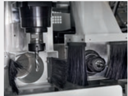
The machine can be equipped with a horizontal and vertical milling unit for making grooves, pockets and slots and for machining Clamex lamello.
