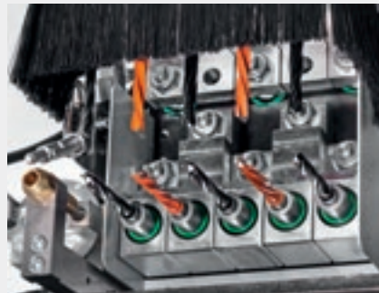
Optional drilling unit fitted with 5 horizontal spindles + 5 vertical spindles.
