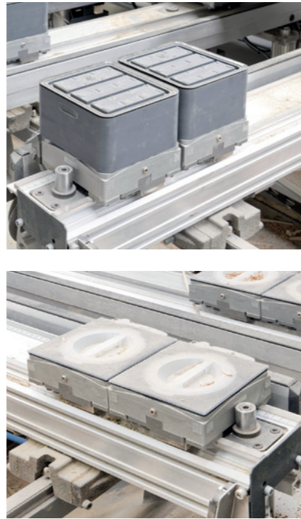
Pop-up stops ensure accurate positioning
