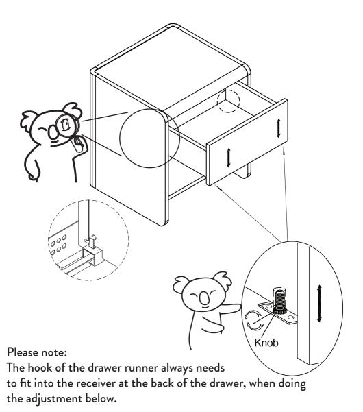
If the drawer's front gap is uneven, you can adjust the drawer front up or down by turning the knob.
