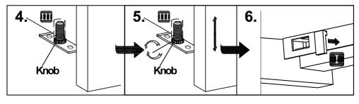
Rest knobs into holes under drawer sides.
