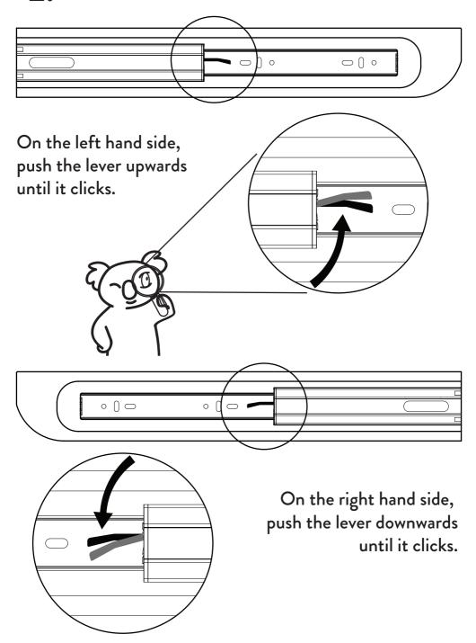
Once the levers are unlocked, pull out the drawer to remove it.
