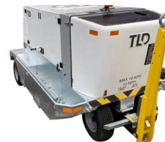
Example of a 90 kVA GPU
