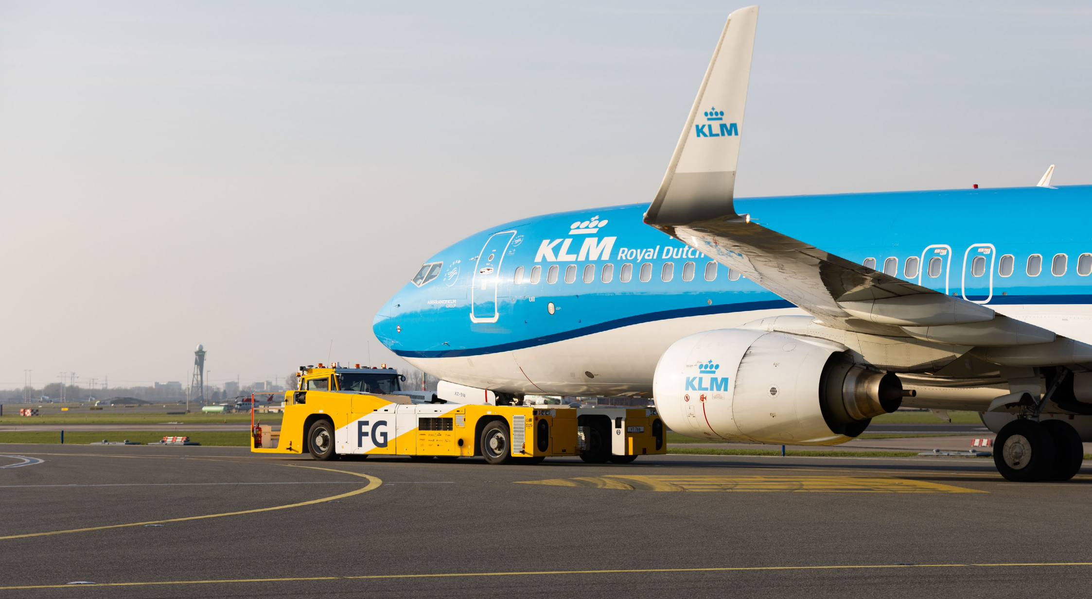
TaxiBot brings the aircraft to the Polderbaan so that the aircraft engines can remain switched off during taxiing.
