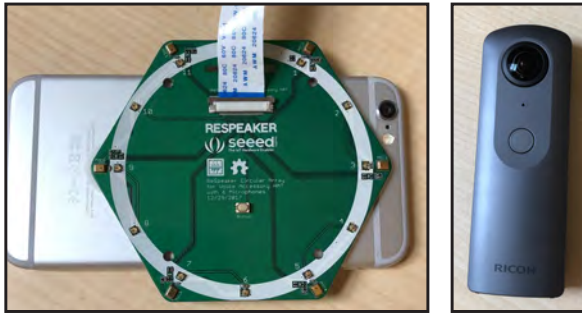
Figure 2: Audiovisual zooming is implemented on two mobile platforms: an off-the-shelf planar microphone array (with 6 microphones) is attached to a smartphone [left] and a 360° Ricoh camera [right] to show smartphone and teleconferencing utility.
