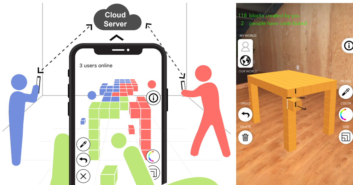
Fig. 2. An illustration of three people co-creating a table in a colocated setup using Blocks (left), and a screenshot showing the Blocks user interface (right). The interface provides functionalities to add a block, pick a color and size, delete or undo blocks, and see collaborators' cursors. Note that Blocks can also be used for remote collaboration when people are not in the same location.
