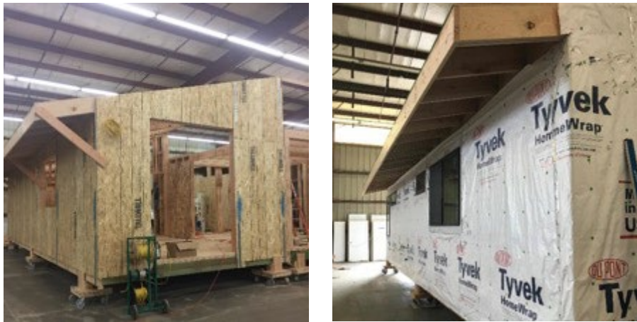
In the factory, the roof is constructed as complete and then separated for shipping.
