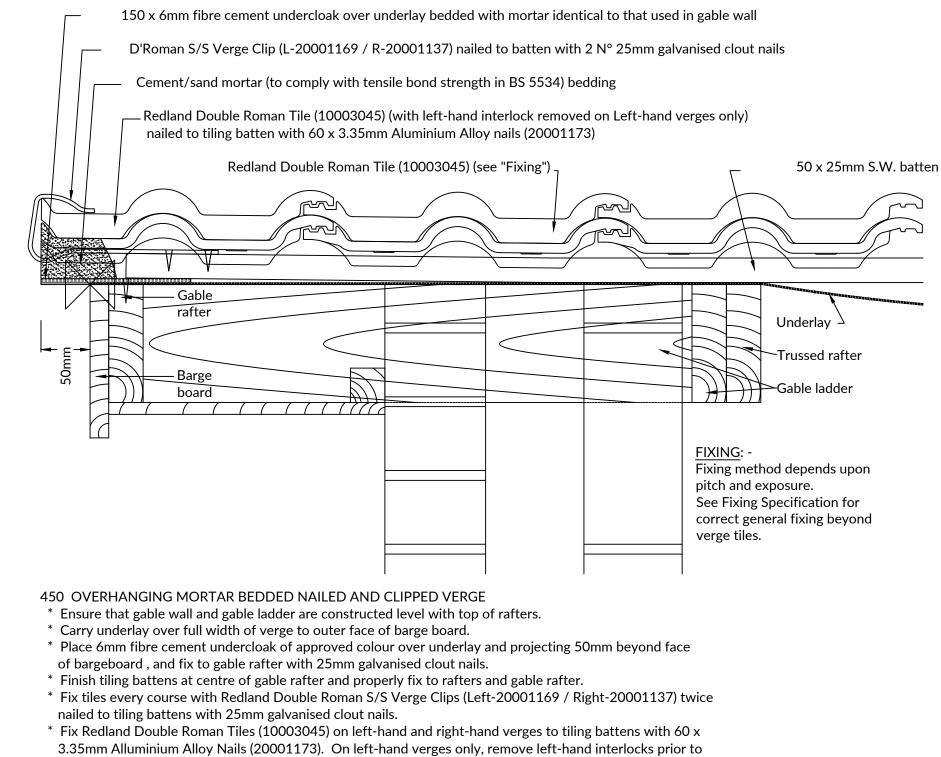
fixing. \* Bed edge of all tiles at verge, on a 75mm wide bed of mortar as clause 290, ensuring that mortar is not displaced or cracked by mechanical fixing of tiles.
