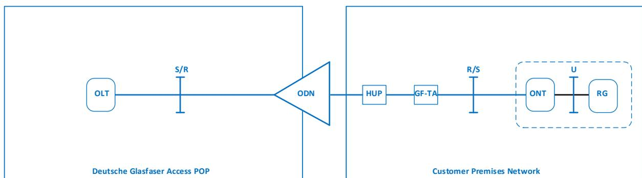
IF<sub>PON</sub> denotes the the interface at reference points S/R and R/S. This interface must support all protocols that are necessary for transmission between OLT and GPON and XGS-PON ONT's/ONU's.
