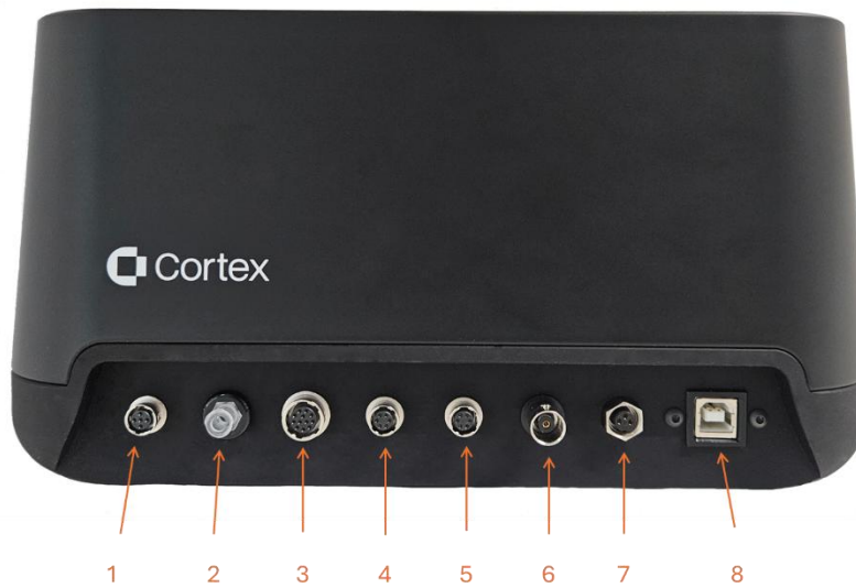
Figure 1. Connectors on the rear panel of the main unit. Table 1 lists how the probes are to be connected to the main unit. Connectors 1 and 2 are for the elasticity probe (both must be connected). Connector 3 is for the ultrasound probe (standard or subcutaneous). Connectors 4 and 5 are for the hydration, skin color, skin temperature, or TEWL probes. Connector 6 is for the pH probe. Connector 7 is for the power supply while connector 8 is for the USB connection to a PC.
