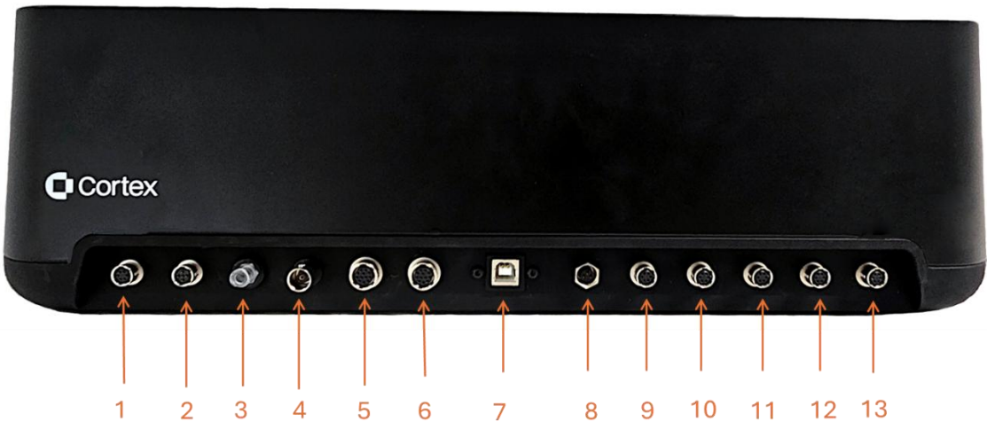
Figure 1: Connectors on the rear panel of the main unit. Table 1 lists how the probes are to be connected to the main unit. Connectors 1, 9, 10, 11, 12 and 13 are universal ports for the hydration, skin color, skin temperature and TEWL probes. Connectors 2 and 3 are for the elasticity probe (both must be connected). Connector 4 is for the pH probe. Connectors 5 and 6 are for the ultrasound probes (standard and subcutaneous). Connector 7 is for the USB connection to a PC while connector 8 is for the power supply.
