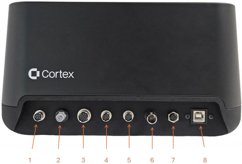
Figure 2. Connectors on the rear panel of the main unit. Table 1 lists how to connect the probes to the main unit. Connectors 1 and 2 are for the elasticity probe (both must be connected). Connector 3 is for the ultrasound probe (standard or subcutaneous). Connectors 4 and 5 are universal ports for the hydration, skin color, skin temperature, or TEWL probe. Connector 6 is for the pH probe. Connector 7 is for the power supply while connector 8 is for the USB connection to a PC.
