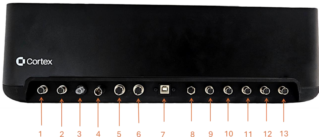
Figure 1: Connectors on the rear panel of the main unit. Table 1 lists how the probes are to be connected to the main unit. Connectors 1, 9, 10, 11, 12 and 13 are for the hydration, skin color, skin temperature, and TEWL probes. Connectors 2 and 3 are for the elasticity probe (both must be connected). Connector 4 is for the pH probe. Connectors 5 and 6 are for the ultrasound probes (standard and subcutaneous). Connector 7 is for the USB connection to a PC while connector 8 is for the power supply.
