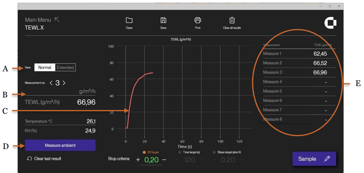
Normal view showing the TEWL measurement in g/m 2 /h (B, C), ambient conditions (D), and history of the latest 8 measurements (E).
