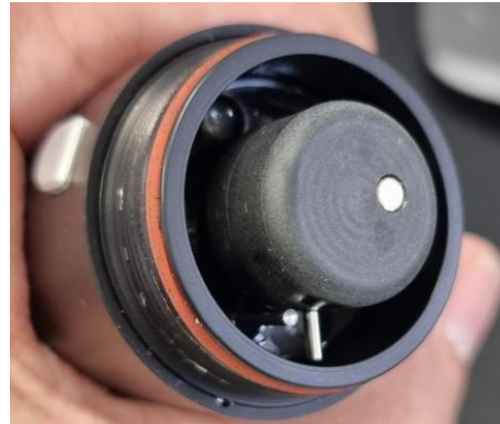
Figure 21 Probe with Button Transducer head
