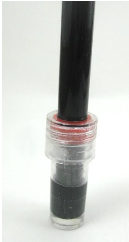
Figure 40 The pH Probe properly stored in buffer solution
