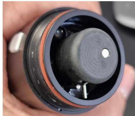
Figure 20 Probe with Button Transducer head
