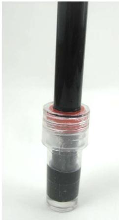
*Figure 42 The pH Probe properly stored in buffer solution*
